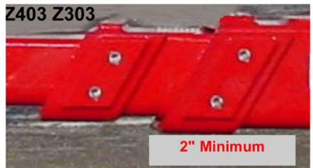
#11) Z403/Z303: Extend middle horizontal extend tube at least 2" from outer horizontal extend tube. This will create an equalization of pressure with inner tube, allowing head to pivot properly during towing. The head will appear to be locked against the inner extend tube but will disengage when turning.
