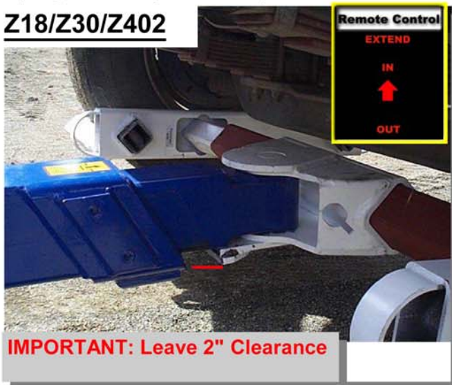
#11) Z403/Z303: Extend middle horizontal extend tube at least 2" from outer horizontal extend tube. This will create an equalization of pressure with inner tube, allowing head to pivot properly during towing. The head will appear to be locked against the inner extend tube but will disengage when turning.
